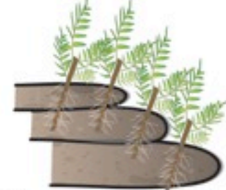
Live revetment uses live stakes and geotextile fabric to rebuild slopes
