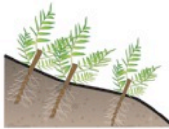
Live stakes, inserted in the ground, establish roots and hold soil in place
